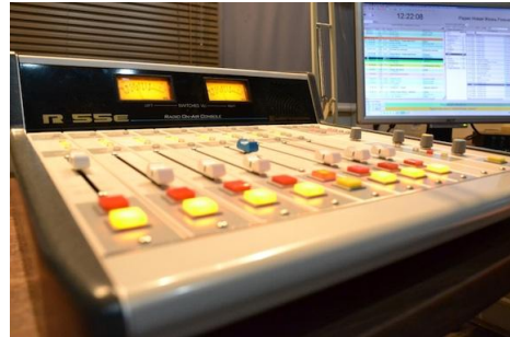
NLR main studio A control center with AudioArts R55 console and Radio Automation system Listen to it at www.NLRadio.net
